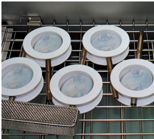
Cleansing the parts with ultrapure water
